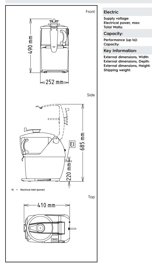
Electric Supply voltage: 200-240 V/1N ph/50/60 Hz Electrical power, max: 1.3 kW **Total Watts:** 1.3 kW Capacity: Performance (up to): 550 kg/hour 5.5 litres Capacity: **Key Information:** External dimensions, Width: 252 mm 485 mm External dimensions, Depth:
